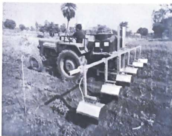
Fig. 3 Field operation of developed shielded sprayer for chilly Data analysis
