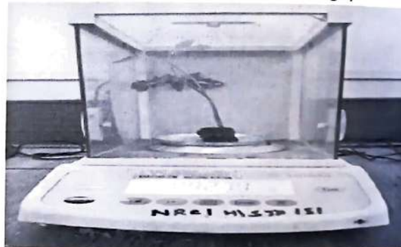
Figure 2 Weighing balance for measuring the plant weight.
